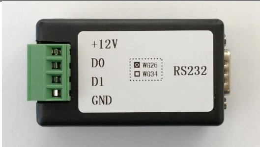
Serial/Wiegand Adapter (Converts Serial/RS232 connection to Wiegand connection)
