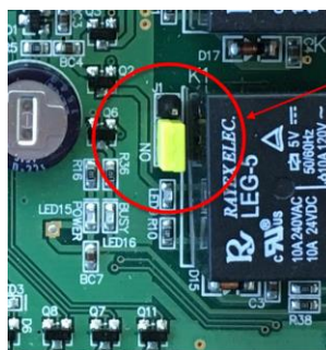
Jumper set to NO (Normally-Open)
