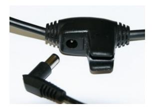
Connect the L-shaped plug of the power supply into the power jack on the barcode scanner cable.
