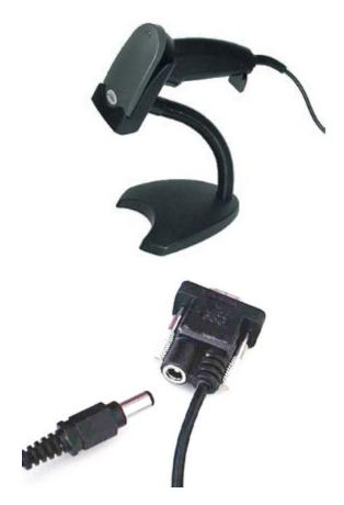
Connect the power supply into an AC outlet.
