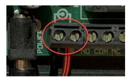
On the Legacy Proximity (Wiegand) Controller, tap 12VDC from the VH and Gnd terminals.
